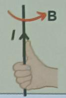
If we hold a current carrying conductor in the grip of the right hand in such a way that thumb points in the direction of current, then curling of fingers represents the direction of magnetic field lines
